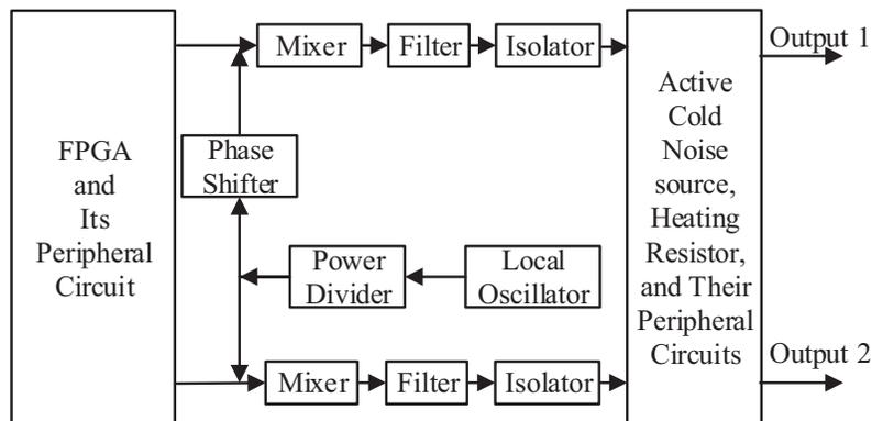
Figure 5: The suggested functional block diagram of the real circuits of actively polarized calibration source.
