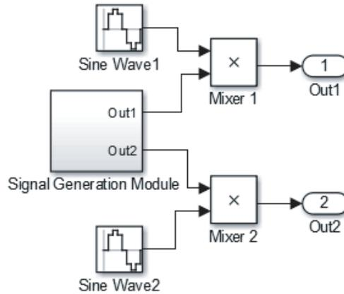
Figure 2: Simulation design of the frequency modulation module.
