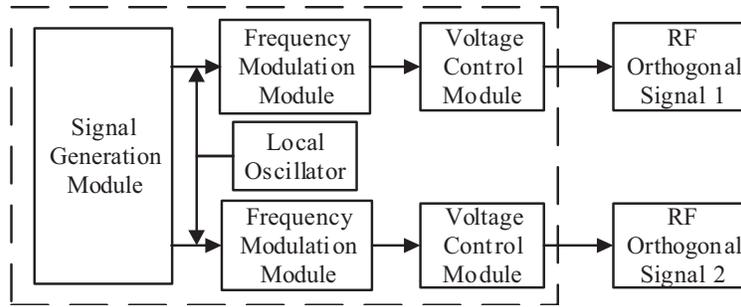
Figure 1: Functional block diagram of the actively polarimetric calibration source.
