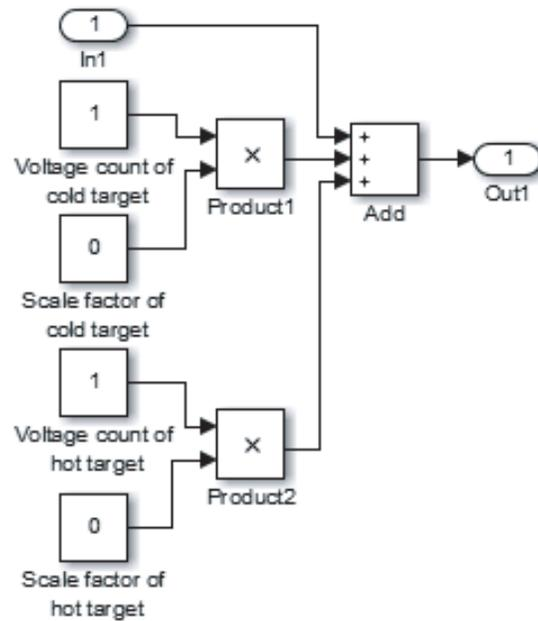
Figure 3: Simulation design of one path in the voltage control module.
