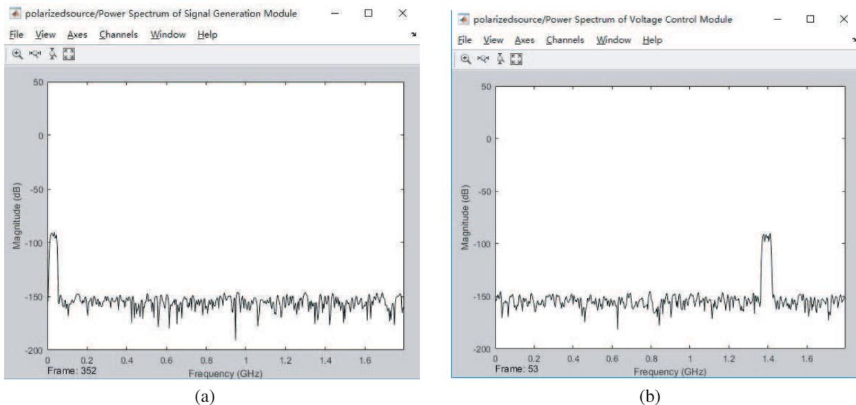
Figure 4: (a) The power spectrum of signal generation module. (b) The power spectrum of voltage control module.
