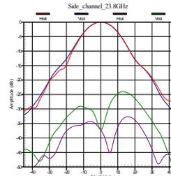
Fig. 7. Patterns of the feed at 23.8GHz frequency
