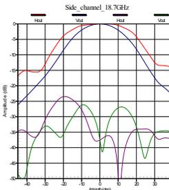
Fig. 8. Patterns of the feed at 18.7GHz frequency
