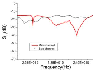
Fig. 5.  $S_{11}$  of the feed with OMT and filters at 23.8GHz band
