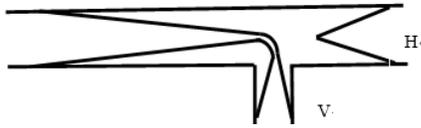
Fig. 2. The Finline OMT connecting with the waveguide.
