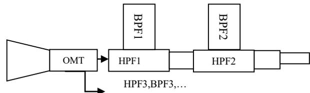
Fig. 1. Diagram of the horn and feeding system
