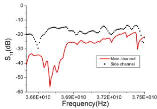
Fig. 3.  $S_{11}$  of the feed with OMT and filters at 37GHz band
