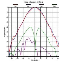
Fig. 6. Patterns of the feed at 37GHz frequency
