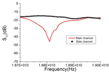
Fig. 4.  $S_{11}$  of the feed with OMT and filters at 18.7GHz band
