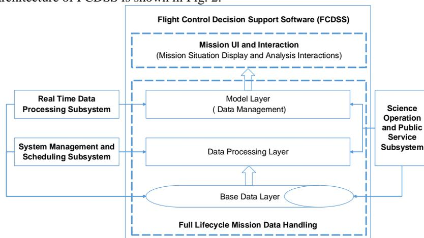
Fig. 2 FCDSS Software Architecture
