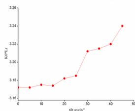
Fig. 5. The resonance length vs offset of the tilt slots.
