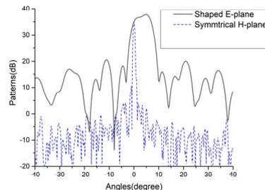
Fig. 6. Shaped patterns in main plane by simulation.
