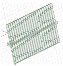
Fig. 2. Diagram of the antenna phase compensation structure.
